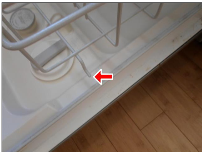
6.10 Item 2(Picture) missing wheels
